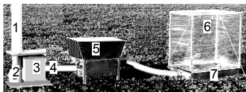
Fig. 1: Canopy chamber system. 1: air supplying tube (only lower part shown); 2: blower; 3: measuring and controlling unit; 4: tube with impeller anemometer; 5: air conditioning unit; 6: canopy enclosure 0.6 m 2 ground area, height 0.8 m or 1.3 m; 7: base frame.
